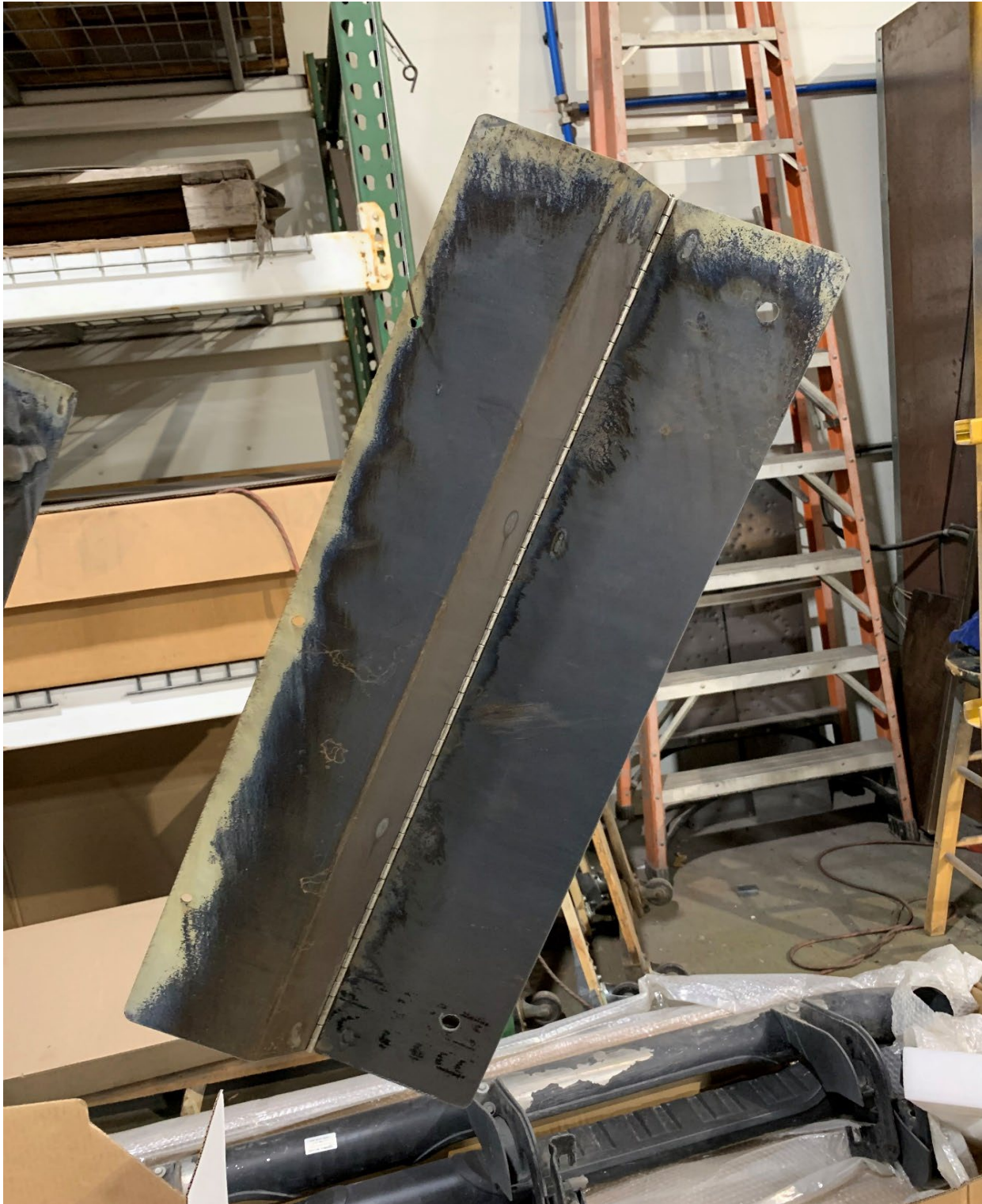
Hot Rolled steel part with mill scale Treated with Picklex® 20 & Oven Dried
