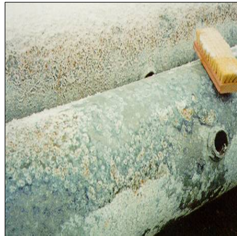
Figure 1: Heavy Wet Storage Stain
