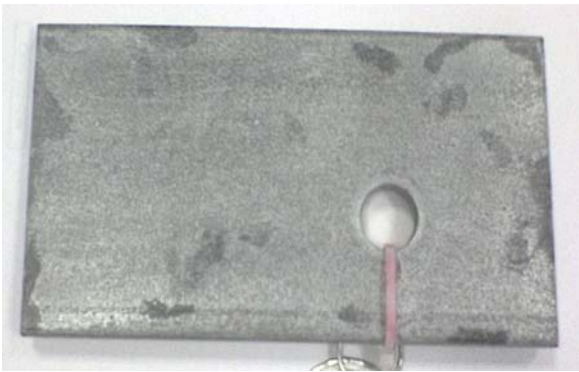
Figure 9: Sample Cleaned with Naval Jelly® Rust Dissolver
