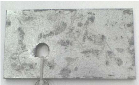
Figure 5: Sample Cleaned with Limejuice
